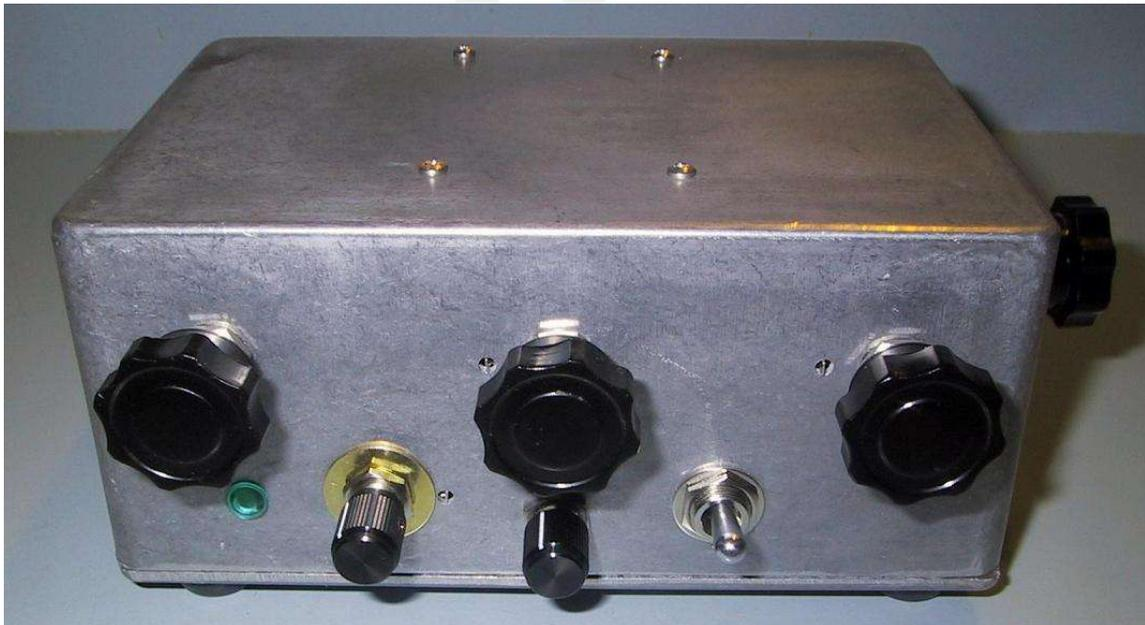
Above is a front panel view of DXP-6-L. The 3 larger knobs from left to right are amplitude 1, phase, and amplitude 2. Previously a 180 degree phase reverse toggle switch for signal path 2 was mounted in that position. The smaller black knob with brass hole reduction washer is one vernier phasing; the other smaller black knob is the other vernier phasing. The toggle switch is a
